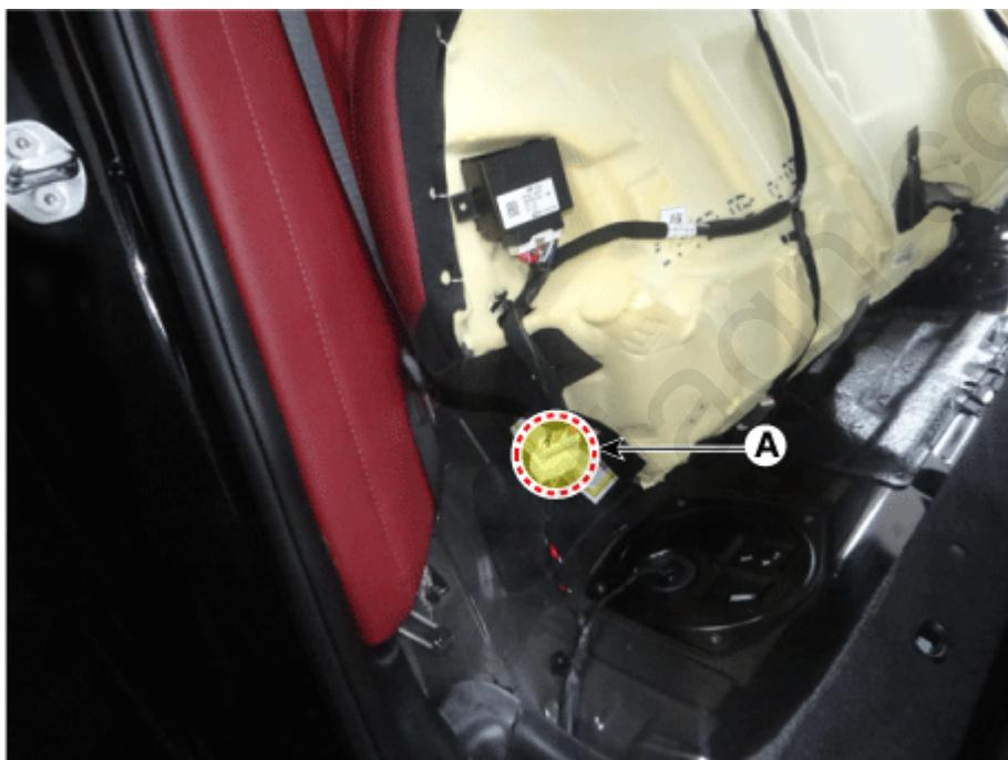
4. Remove the rear back side seat (A) by pulling it up after loosening the mounting bolts.
