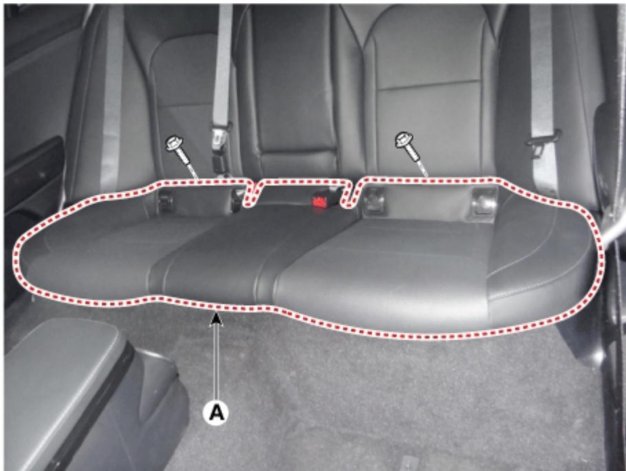
3. Remove the rear seat cushion after disconnecting the heater connector (A).
