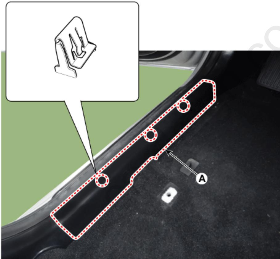
2. Separate the rear seat cushion (A) after loosening the mounting bolts.
